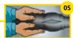
05 Joining Izocamflex starting from the ends
