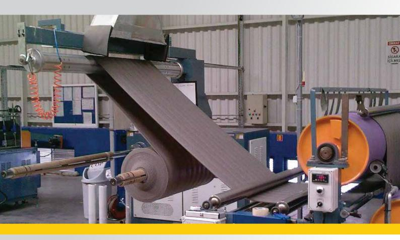
Polyethylene is a flexible thermal insulation material that has closed porosity and even cell structure. It can be manufactured in the forms of sheet, pipe and cord in different size and with different technical properties and varied facing materials according to the intented use and the place of use. It is used for thermal insulation and condensation control.
